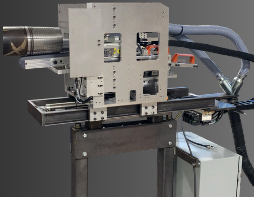
Automated Pipe Cleaning System
