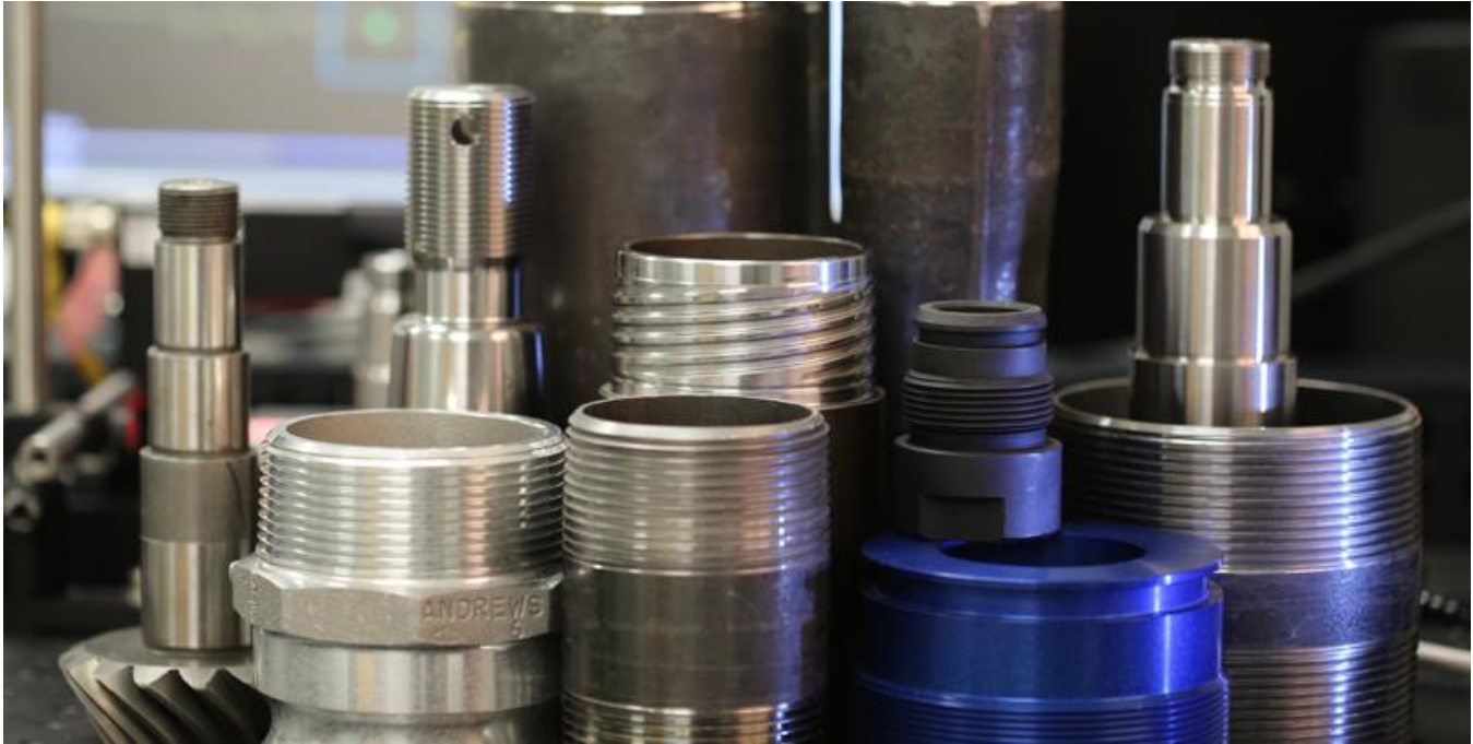
Figure 1: Example of work pieces gauged using Autonetics SGU
