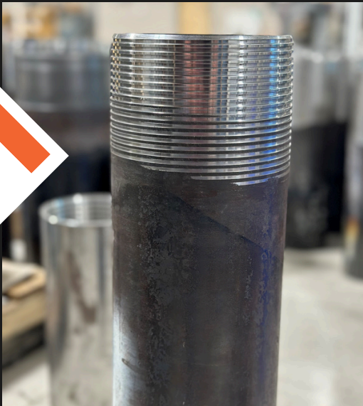
Buttress Threaded Connection
